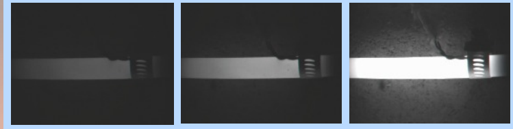
Actual VIS ThermalVision™ Camera measuring rod Temperatures 750°F [400°C] - 2865°F [1575°C]
