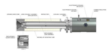
Similar to the UltraTemperature camera, a positive air flow runs over the lens in order to keep the optics clean, and also provides lens cooling in this case, with a typical air flow path seen below.
