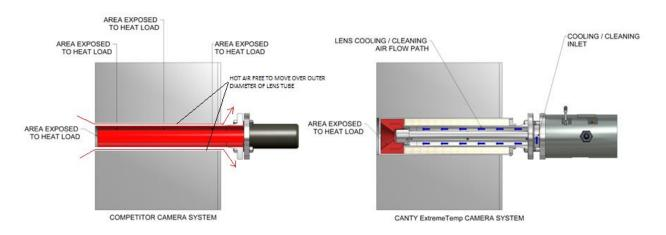
It is due to this type of installation that the lens of the retractable type camera systems require constant air cooling, and have issues of instantaneous component failure should the air supply fail.
