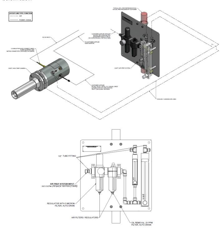
In an ExtremeTemperature camera, if the cleaning / cooling air fails, there is no instantaneous failure of any components. If the process is operating close to the camera specification upper limit of 1650C, the user will have sufficient time (~2 hours) to either get the air supply up and running again, or to manually remove the camera system from the process.
