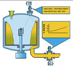
The Canty Camera / Light combination views the liquid centrate discharge from the centrifuge to determine color, % solids and broken particulate, and provides the 4-20mA output required for continuous control.
