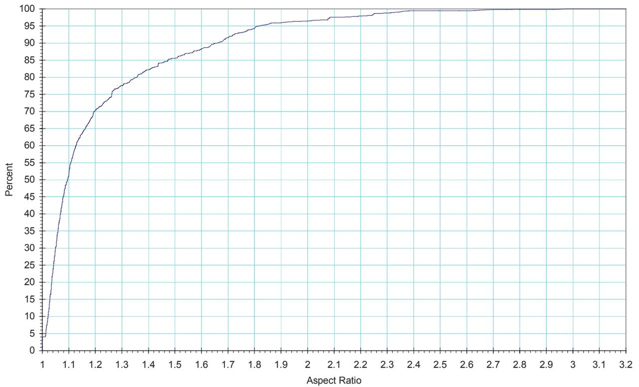
Figure 9, Medium Material Aspect Ratio Distribution by Volume Percent Passing
