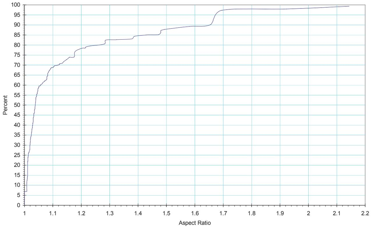
Figure 12, Coarse Material Aspect Ratio Distribution by Volume Percent Passing
