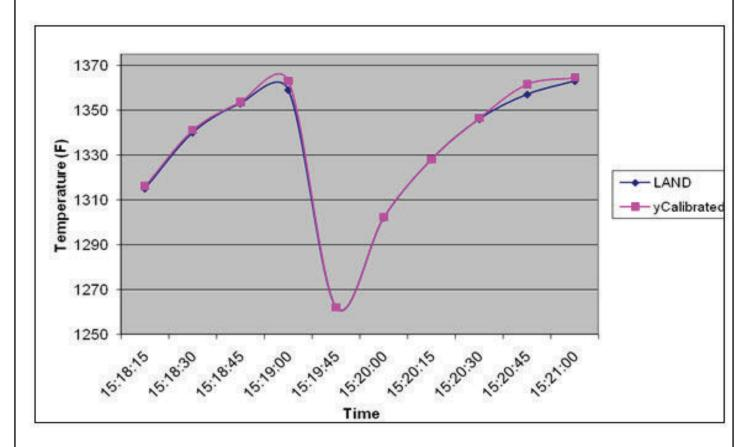
The camera readings consisted of the y value of the color space, more commonly known as the intensity. As can be seen from the graph the two curves match quite closely. This result is expected for most cases as both technologies measure the intensity of various wave length segments over the electro magnetic spectrum.
