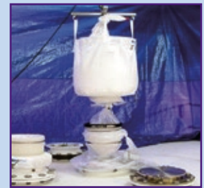
Vessel Charging and Sampling with Dover Pac®
