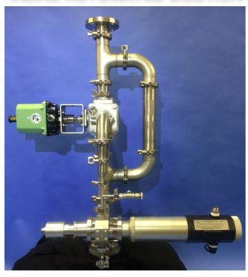
Combining the latest in CCD Ethernet camera technology with Canty fused glass, lighting and CANTYVISION $^{\text{TM}}$  software, the INLINE AUTOMATED DILUTION PARTICLE SIZE Measurement System provides real time In Flow measurement of particulate in a slurry.
