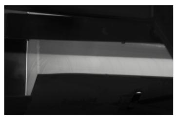
The image to the left has been taken with a Canty camera optimized for glass edge measurement. The graph below shows the strength of the edges along a line going from left to right on the image. This is what is used to detect the primary glass edge. Notice there is little to no noise.
