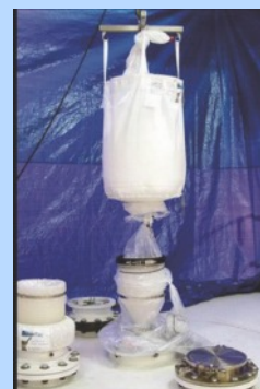
Vessel Charging and Sampling with Dover Pac®
