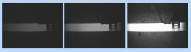
Actual VIS ThermalVision™ Camera measuring rod Temperatures 750°F [400°C] - 2865°F [1575°C]
