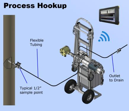
The Transportable INFLOW<sup>™</sup> is designed for multi point site surveys, and testing or trouble shooting of any oilfield separation systems.
