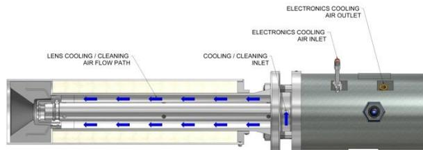
Note that the electronics cooling air is a common requirement for Canty and retractable type systems, and does not have any influence on whether a retraction system would be required or not.
