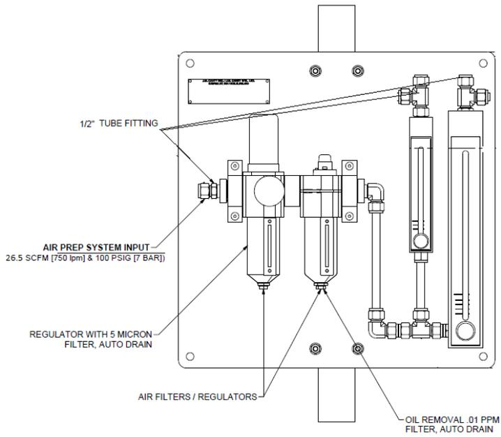
In an ExtremeTemperature camera, if the cleaning / cooling air fails, there is no instantaneous failure of any components. If the process is operating close to the camera specification upper limit of 1650C, the user will have sufficient time (~2 hours) to either get the air supply up and running again, or to manually remove the camera system from the process.
