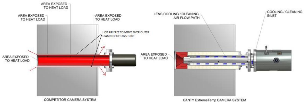
It is due to this type of installation that the lens of the retractable type camera systems require constant air cooling, and have issues of instantaneous component failure should the air supply fail.
