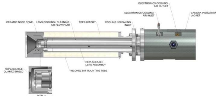
Similar to the UltraTemperature camera, a positive air flow runs over the lens in order to keep the optics clean, and also provides lens cooling in this case, with a typical air flow path seen below.
