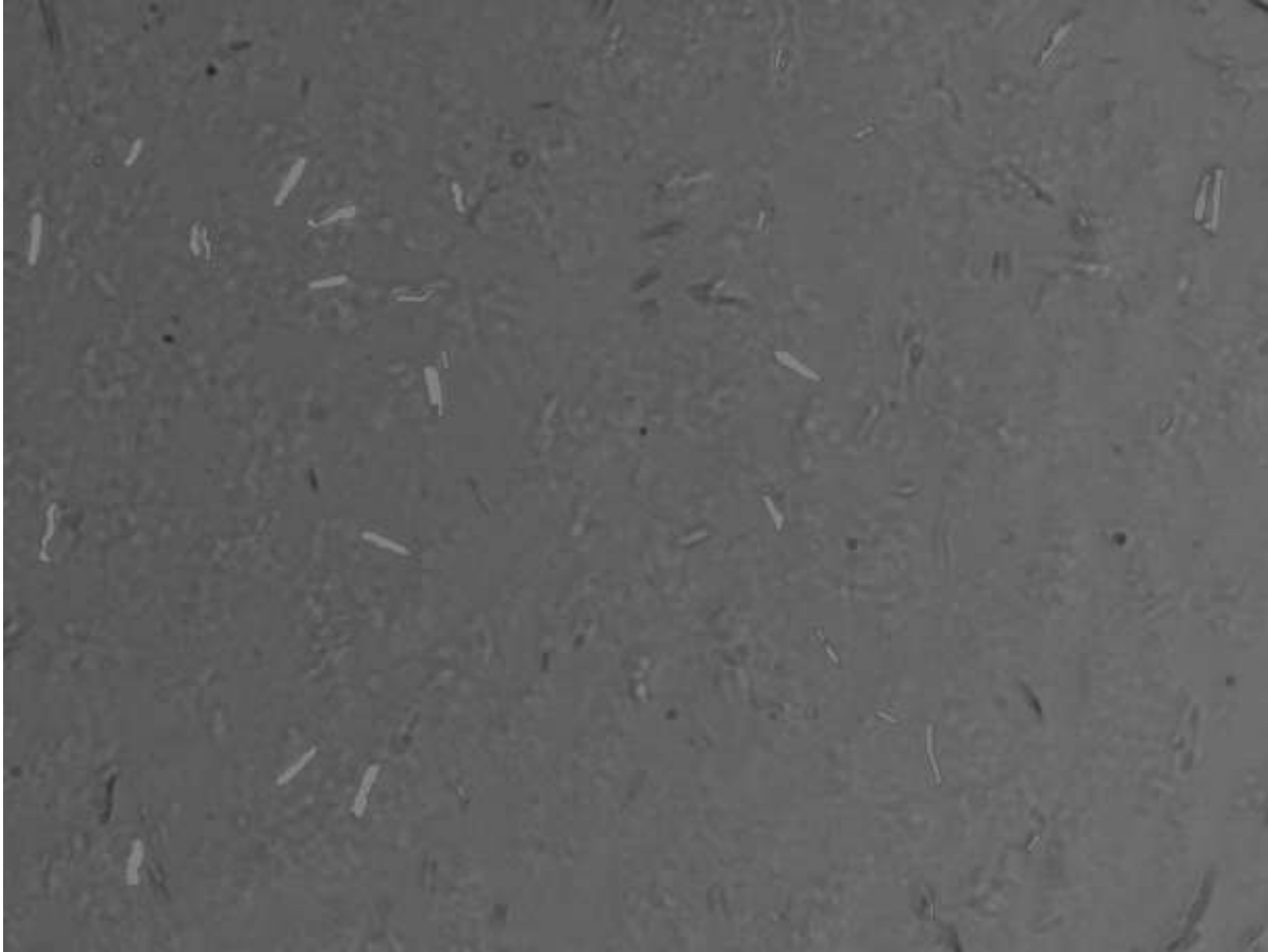
Figure 2 – 2% Wax in Oil analyzed using Canty Vision Particle Sizing Sizing Software
