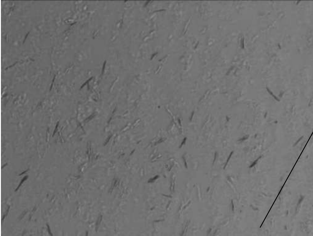
Figure 5 – SAM2517- Wax particles aligning in direction of flow
