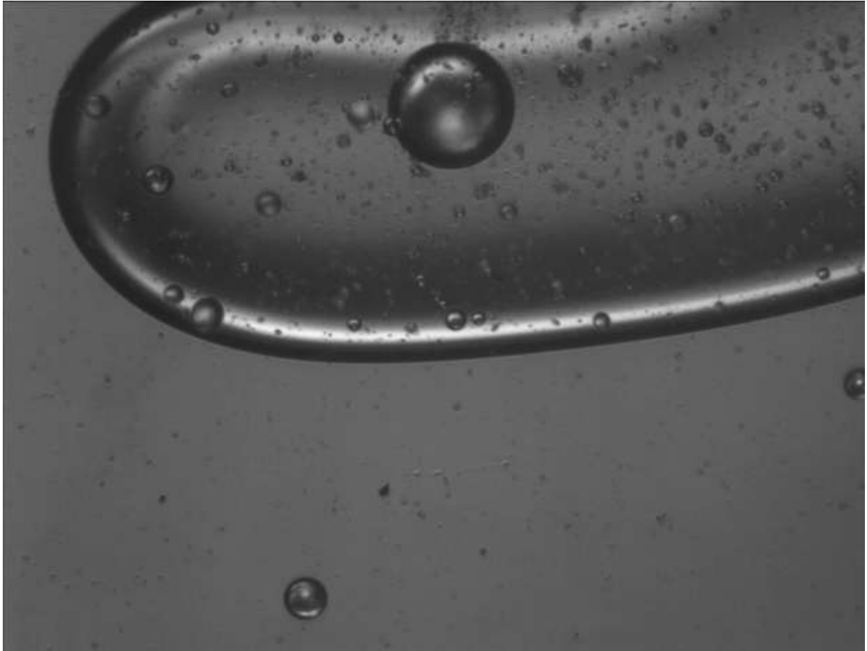
Figure 3 - A large slug of material is seen as the valve is opened and the interface change is occurring in the flow cell.
