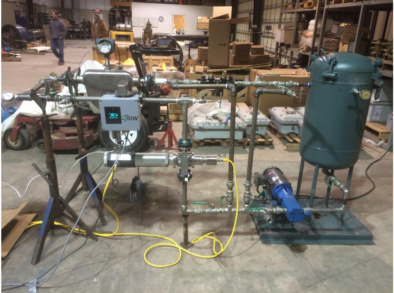
Figure 1-Flow Loop Setup, Star Measurement Lafayette LA
