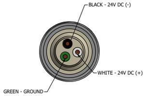
INPUT WIRING SCHEMATIC
