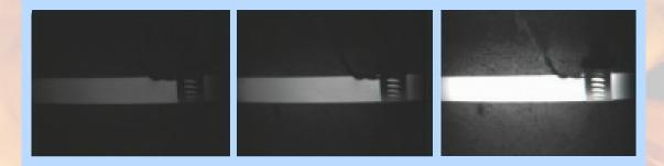
CANTY provides continuous temperature measurement by using multiband wavelength imaging pyrometry. With the advancement of CCD technology, multiband measurement has several advantages over 2 color (2 wavelength) pyrometers:
