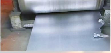
CANTY cameras can identify smooth vs wavy edges, with wavy edges potentially causing downstream problems that can be prevented through prompt corrective actions. Additionally, CANTY cameras can spot holes and tears in the strip, triggering CANTY software alerts for operators to take corrective measures before incurring expensive downtime.
