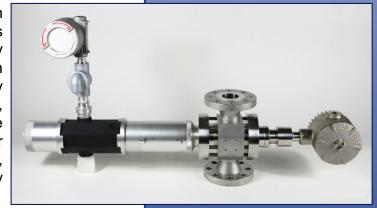
The Canty Inflow works on the premise of dynamic imaging. It is installed inline with process flowing through it. As particles are detected, the Inflow will quantify the size and concentration of the polymer and output these values as tags to a control system. This system can then be set up to alert personnel of the problem and even begin measures to mitigate the situation.
