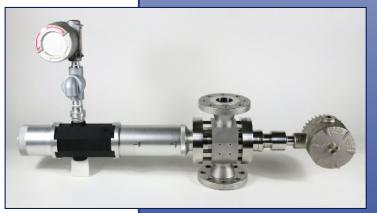
The Canty Inflow works on the premise of dynamic imaging. It is installed inline with process flowing through it. As particles are detected, the Inflow will quantify the size and concentration of the polymer and output these values as tags to a control system. This system can then be set up to alert personnel of the problem and even begin measures to mitigate the situation.
