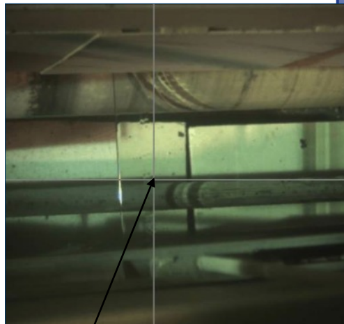
Inner Knurl Edge Tracked by CantyVision™ (note cross-hair position)
