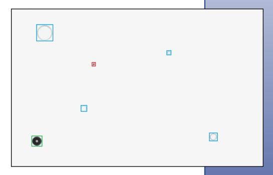
After a particle has been sorted into its correct class, the software calculates a volume of that particle based on its class. Since we already have the volume of each image being analyzed, the concentration of any given class of particle can now be calculated on a volumetric basis and can be converted into a mass concentration using the bulk density of the particle class in question.
