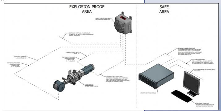
CAT6 Ethernet, however, has a distance limitation of 100m before there is signal loss that can interrupt analysis. In those situations, it is possible to convert the CAT6 Ethernet to fiber via CANTY's media converters. Refer to document TA11950-1024. Using this method, it is possible to run a fiber line up to 10km between the analyzer's power supply and then VCM. In this case, a typical layout of the components will look like the following.
