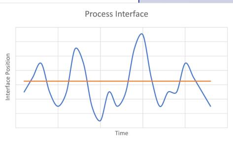
Once an interface has been detected, the software then calculates the position of that interface in pixels, converts it into a real-world value, and outputs that value via a number of different available control signals.
