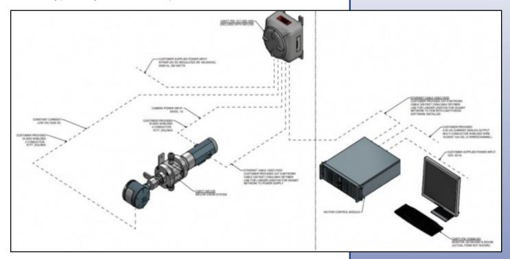
Ethernet, however, has a distance limitation of 100m before there is signal loss that can interrupt analysis. In those situations, it is possible to convert the Ethernet to fiber via CANTY's media converters. Refer to document TA11950-1024. Using this method, it is possible to run a fiber line up to 10km between the analyzer's power supply and then VCM. In this case, a typical layout of the components will look like the following.
