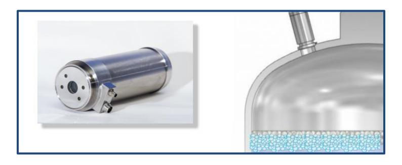
Automation of these antifoam inputs can thus reduce downstream processing and mitigate the risk of over foaming. The Canty technique replaces the visual inspection with an automated live image achieved with a camera. Canty foam control operates using a vision based principle to capture live images of the process as foam is forming. The Cantyvision software suite uses advanced image processing techniques to detect light reflection from the bubbles of the foam itself.
